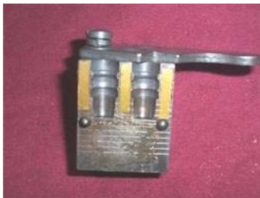
358429 that was undersized in all dimensions This coverage by .002" brass stock brought even the front band to full diameter.
