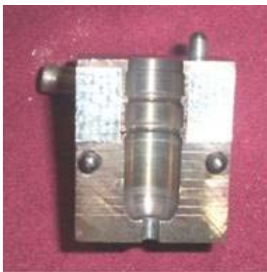
462560HP enlarges to .461" This mould had a loose gas check also.
