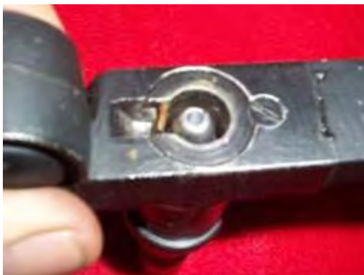
Figure 2: Inserting the bullet in the die
