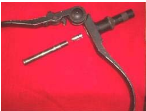
Figure 1: 310 tool set up with die installed. Push rod and bullet are positioned for insertion of bullet
