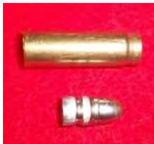
Top: Home made Kakecutter Bottom: Sized 358311 bullet
