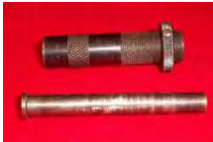
Ideal Sizer Die Assembly Top: Sizer Die (.358) Bottom: Push Rod (#311 for bullet #358311)
