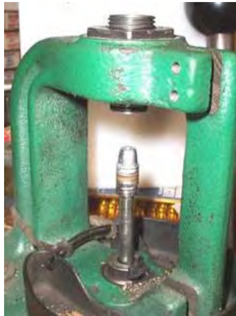
Nose first sizer with bullet ready for nose first sizing (In this case, I'm downsizing a bullet that has already been sized and lubed)
