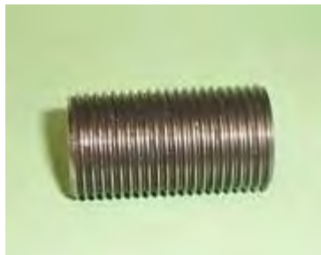
7/8 X 14 die body opened to .700" and cut to 2" to accept Lyman/RCBS sizers
