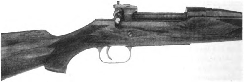
Fig. 13 Side view of Ross rifle action, bolt closed
