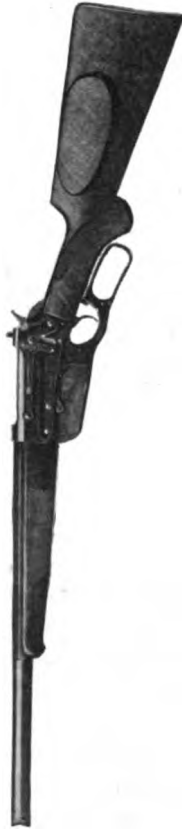
Fig. 6 A special Winchester Model 1895 rifle belonging to the author, and used by him for a number of years. Caliber .40-72, heavy No. 3 half-octagon barrel, and hand-made, pistol-grip stock.
