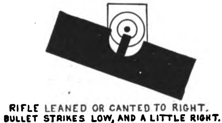
Fig. 113 Showing errors of aim, and the result
