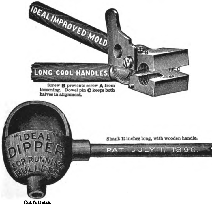
Fig. 83 Ideal bullet mould and dipper
