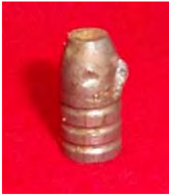
457122 HP “whisper” bullet recovered at 100 yards. Took a few dings but is mainly intact.
