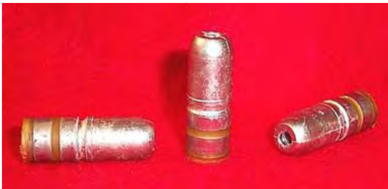
From Left: 462560 and 462560 HP "Solid" is 549.0 grains Hollow point is 532.1 grains
