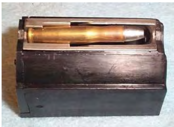
Ruger Hornet Magazine showing bullet fit #225415 HP loaded to Lyman Cast Bullet Manual length
