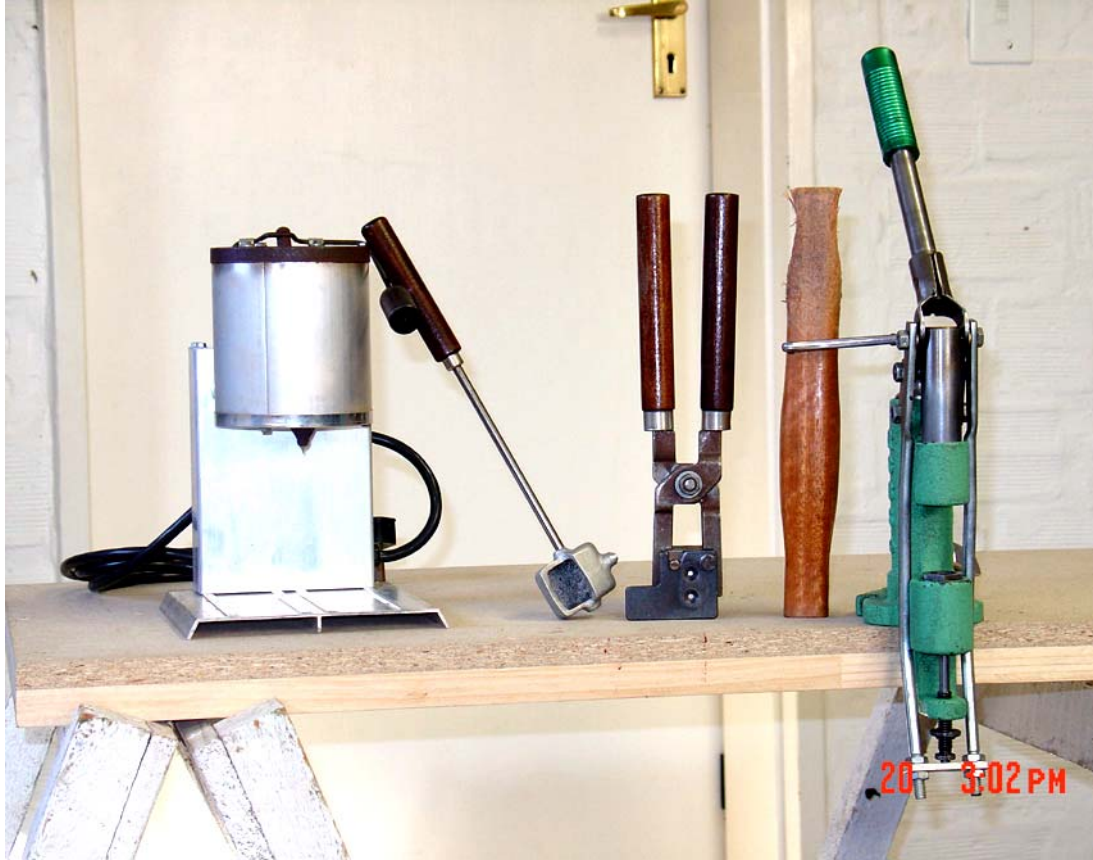
Fig 3 Lee melting pot, RCBS dipper, RCBS mould and handles, hammer shaft for use as mallet, and RCBS
