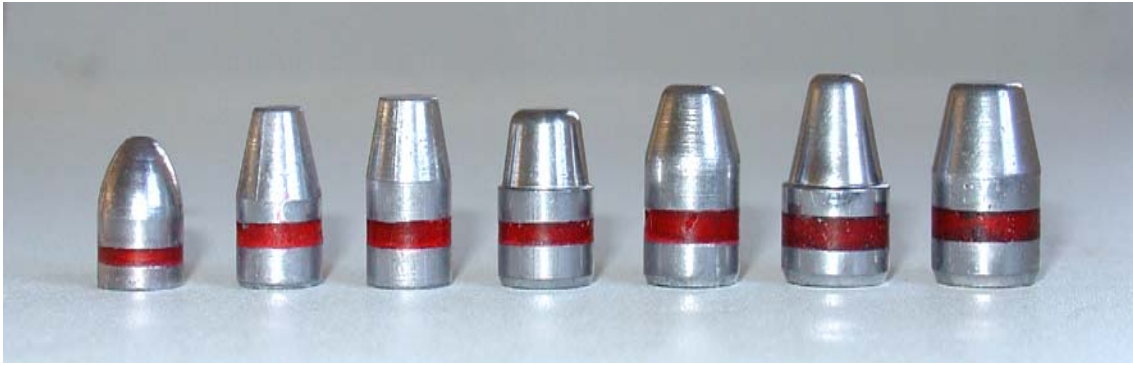
Lee 100 grain 380 Auto, Lee 120 grain 9mm, Lyman 130 grain 9mm, Lyman 150 grain 40 S&W, Magma 180 grain 40 S&W, Lee 200 grain 45 ACP, Lee 230 grain 45 ACP.
